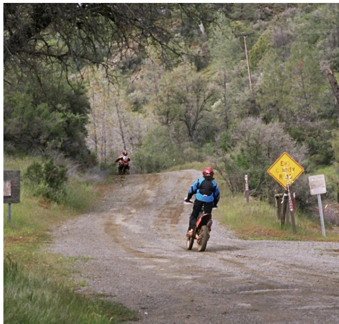
Figure 1. The lead rider in the EPA Region 9 study is shown to be generating a large dust cloud to which the trailing rider is exposed. By comparison neither the lead nor trailing IERF riders are generating visible dust during the April, 2010 activity based air sampling, the airborne asbestos exposure for both IERF riders is statistically identical. Asbestos exposure to the EPA Region 9 trailing rider is about 20-fold higher than the two IERF riders.
